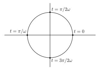
The velocity  $\mathbf{v}(t) = (-r\omega \sin \omega t, r\omega \cos \omega t)$  has constant length  $v = r\omega$ , and likewise the acceleration  $\mathbf{a}(t) = (-r\omega^2 \cos \omega t, -r\omega^2 \sin \omega t)$  has constant length  $a = r\omega^2$ . In turn this implies the relation
